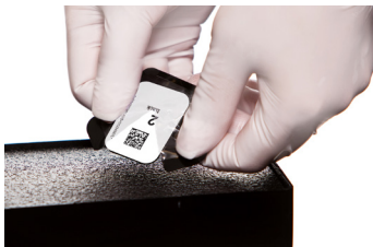
View B: Ejecting imaging plate to transfer box
