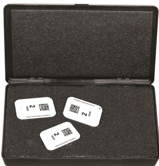
View C: Imaging plates ready for Scanning
