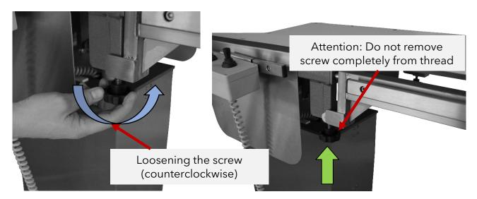
Thereafter, the relevant frame half can be easily pulled out of the construction and detached from the table.
