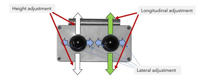
The height adjustment, longitudinal adjustment and lateral adjustment are performed by electronic actuators. By the joysticks in the above-mentioned directions, the height adjustment as well as the longitudinal and lateral adjustment are carried out.
