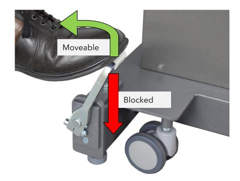
The product can be locked in the designated position by means of blockable rubber feet. This mechanism is activated by pressing one of the two levers at the head or foot end of the tabe base. To ensure a stable stand, the rubber feet need to be locked at both ends.
