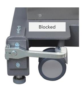
Pressing down one of the two locking levers on the front side of the base frame, respectively bringing it into the horizontal position, will extend the installed rubber feet to stabilize and secure the product. As a result, the product table can no longer be maneuvered.
