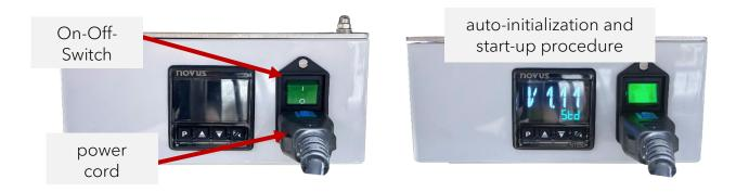
Hence, the unit initiates a self-test to check its functions. Subsequently, the memorized program is executed.
