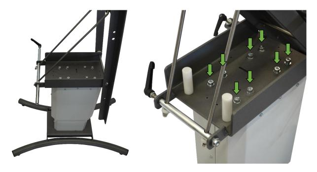
Subsequently, fix the top with delivered screws (8pcs. M8) as well as corresponding washers into the 8 screw holes from above with the assistance of a 6 mm Allen key, as shown in the picture instructions above. Please note that if different screw types are included in your scope of delivery, the stronger/thicker screws (larger diameter) are required to be appropriated in the given context.
