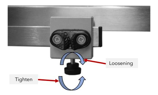
Prior to use, the accessory has to be loosened at the respective locking screw and threaded laterally onto the siderail. Once the desired position of the tie-down cleat on the rail has been attained, it must be tightened at the locking screw to stabilize it in place.
