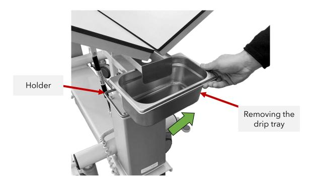
The drip tray can be easily detached from the corresponding holder - e.g. for emptying and cleaning - (by first pulling it upwards and then slightly to the side to prevent it from colliding with other parts of the table) or reinserted (in reverse order) as well as reconnected to the table.
