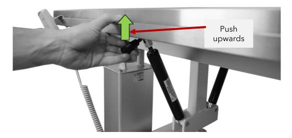
For each half of the table top, the lever on the respective gas pressure spring must be pushed upwards. Hold the lever in position and maneuver the respective table top half until the desired angle of tilt is reached. The gas spring support should enable the upward movement of the table top to be carried out fairly comfortably, while the downward movement requires additional assistance from the user.
