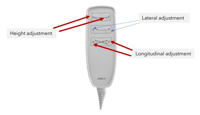
The height adjustment, longitudinal adjustment and lateral adjustment are performed by electronic actuators. By pressing the above-mentioned buttons on the hand control, the height adjustment as well as the longitudinal and lateral adjustment are carried out.
