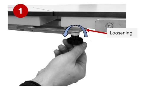
After loosening both locking screws (left and right!), the corresponding laparoscopy cut-out can be pulled out of the table top in parallel to the plate surface for removal. It is advisable to use both hands to detach the cut-out from the device parallel to the two fixation points (near the locking screws).
