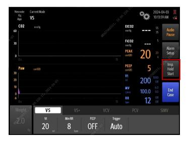
4. As needed, select the [Min Delay Time] and [Duration Time]. After setting, click  $[\sqrt{\ }]$ :
