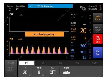
6. The screen will subsequently display 【Insp. Hold Active】 and be accompanied by an alarm sound:
