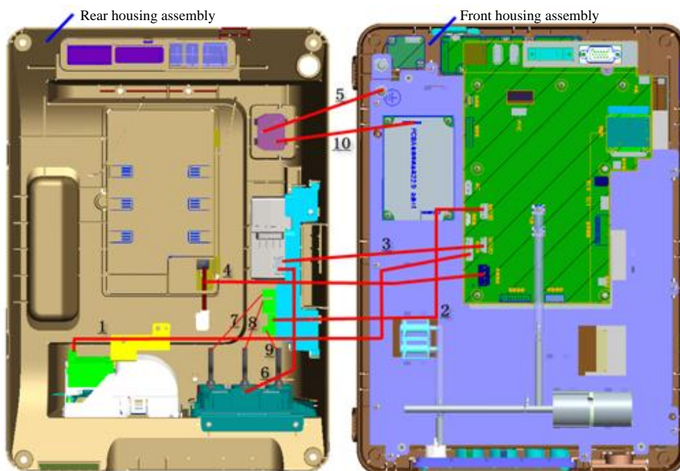
Figure 6 Front and rear housing cabling
